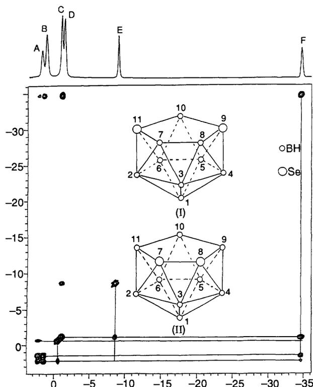
Figure 9 An  $^{11}\text{B}$  COSY experiment on  $[\text{B}_9\text{H}_9\text{Se}_2]$  carried out at 14.1 T.
