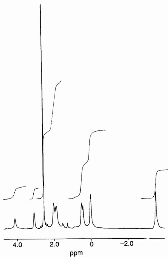
Figure 14 360.13 MHz  $^1\text{H}\{^{11}\text{B}\}$  NMR spectrum of  $[\text{B}_9\text{H}_{13}\text{SEt}_2]$  (8.46 T).
