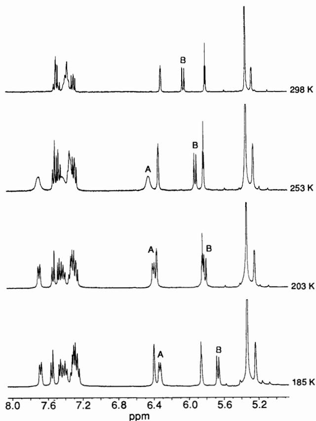
Figure 17 Variable temperature  $^1\text{H}$  NMR spectra of  $[1\text{-Ph-}3\text{-(}\pi\text{-C}_9\text{H}_7\text{)-}3,1,2\text{-closo-CoC}_2\text{B}_9\text{H}_{10}]$ .
