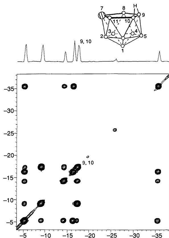
**Figure 7** An  $^{11}\text{B}$  COSY Experiment on  $[\text{B}_{10}\text{H}_{11}\text{Se}^-]$ , carried out at 14.1 T.
