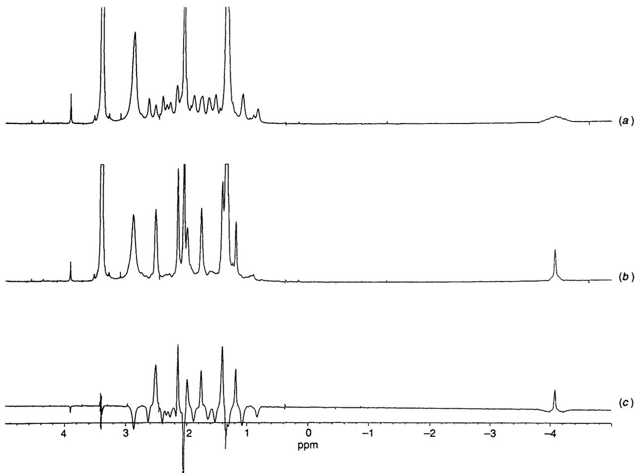
**Figure 2** (a)  $^1\text{H}$  spectrum of  $[\text{NEt}_4][\text{B}_{10}\text{H}_{11}\text{Se}]$ ; (b)  $^1\text{H}\{^{11}\text{B}\}$  spectrum of  $[\text{NEt}_4][\text{B}_{10}\text{H}_{11}\text{Se}]$ ; (c) (b) - (a).
