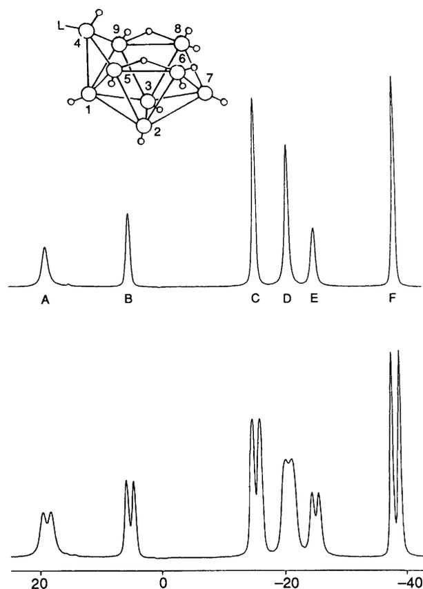
**Figure 12** 115.5 MHz  $^{11}\text{B}$  (bottom) and  $^{11}\text{B}\{^1\text{H}\}$  (top) NMR spectra of  $[\text{B}_9\text{H}_{13}\text{SEt}_2]$  (8.46 T), and its structure.
