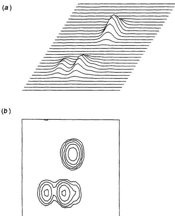
Figure 4 Examples of (a) a stacked plot two-dimensional spectrum and (b) the same data presented as a contour plot.
