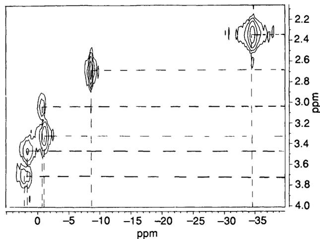
Figure 5 An  ${}^{11}B/{}^1H$  two-dimensional correlation experiment on  $[B_9H_9Se_2]$  carried out at 8.46 T (360.1 MHz for  ${}^1H$ ; 115.5 MHz for  ${}^{11}B$ ).
