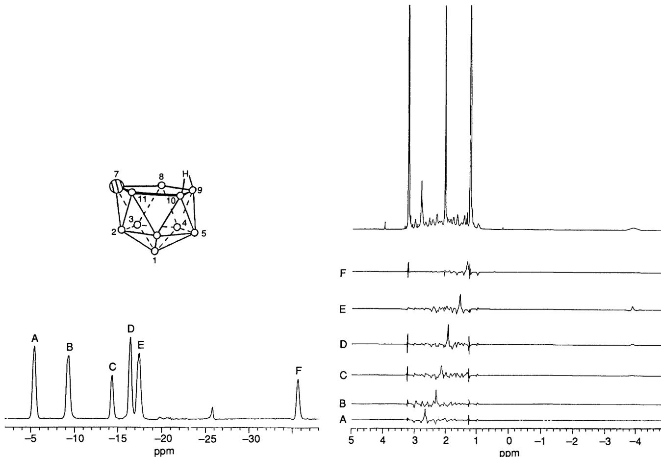
**Figure 6** A series of selective  $^1\text{H}\{^{11}\text{B}\}$  difference spectra for  $[\text{B}_{10}\text{H}_{11}\text{Se}^-]$ , carried out at 14.1 T. An  $^{11}\text{B}\{^1\text{H}\}$  spectrum shows the  $^{11}\text{B}$  decoupling sites.
